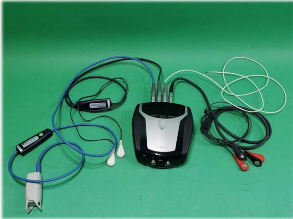
Slika 21 – Nexus 10 uređaj (izvor slike https://www.dotmed.com/listing/other/nexus/mindmedia-10-mkii-mark-2/neurofeedback-biofeedback-emg-system/4957007 )
