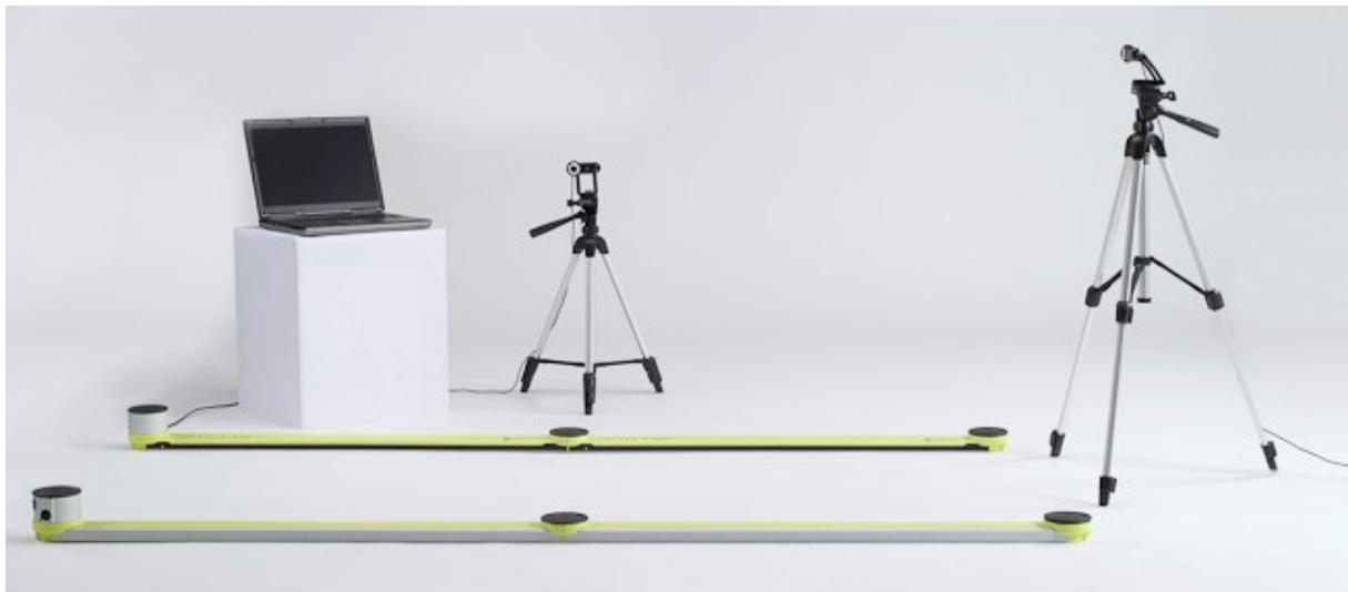
*Slika 4. Optojump next sustav (Slika preuzeta sa <http://www.optojump.com/What-is-Optojump.aspx>)*
