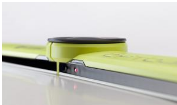
Slika 9. Optojump mjerni instrument (preuzeto sa: http://www.optojump.com/What-is-Optojump.aspx )
