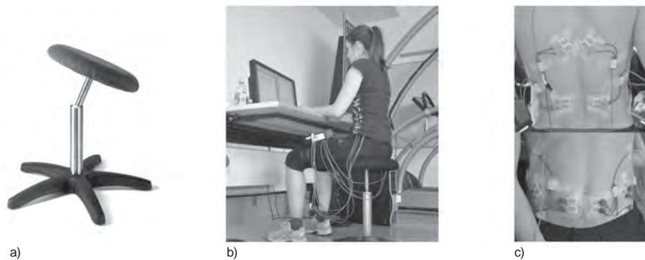
Figure 1: Representation of a) a novel chair with unstable seat (Active Chair ® ), b) a computerized office task while measuring EMG activity on the Active Chair ® and c) EMG electrodes positions for left and right lower trapezius and erector spinae (upper picture) and rectus abdominis and obliquus externus (lower picture) muscles.
