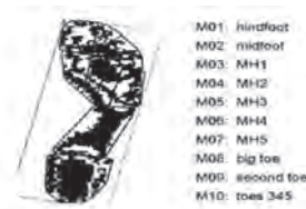
Figure 3: Division of the sole into areas
