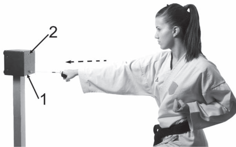
Figure 1. Measurement setup example. 1 = linear position sensor (LPS) and 2 = four LED lights on the LPS. The participant had to react on the light stimulus and make an offensive action (reverse hand punch) against the LPS. Picture is symbolic.
