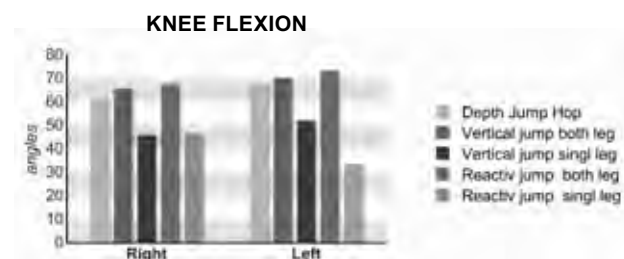
Figure 3. Knee flexion during the maximal vertical jump, the reactive jumps and the drop-jump
